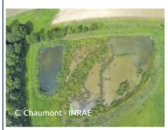
In 2010, four artificial buffer wetlands were created in a 355-hectare agricultural catchment area. They were equipped with instruments to monitor their effect on pollutant flows over time. The four wetlands represent 0.2% of the total area of the drained basin.
