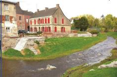
In order to reduce the risk of floods in the municipality, the river has been restored and two weirs have been removed to slow down the flow upstream of Hirson, increasing the storage capacity of the river bed during floods.
