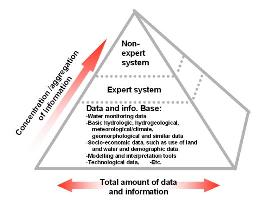
**Figure 5.** Schematic illustration of the generally accessible Environmental Information system (EIS) including a data and information base that contains core data, an expert system for users with necessary knowledge, and a highly aggregated and easily understandable non-expert system.
