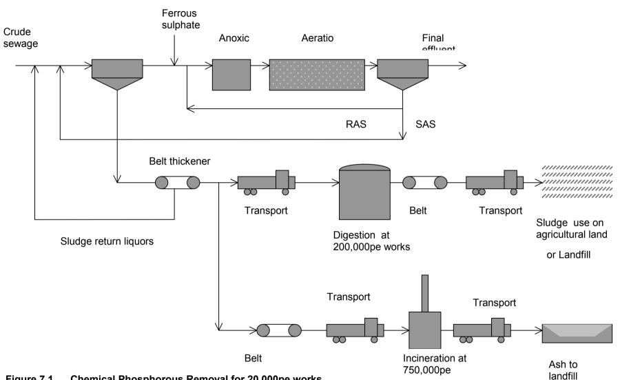
Figure 7.1 Chemical Phosphorous Removal for 20,000pe works
