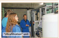
Membrane manufacturers participated in this pilot unit with 2 modules that are already operating (Aquasource and Polymem) and two others that will be installed later (X-flow and Hydranautics).
